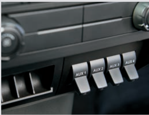
Standard upfitter switches on diesel
