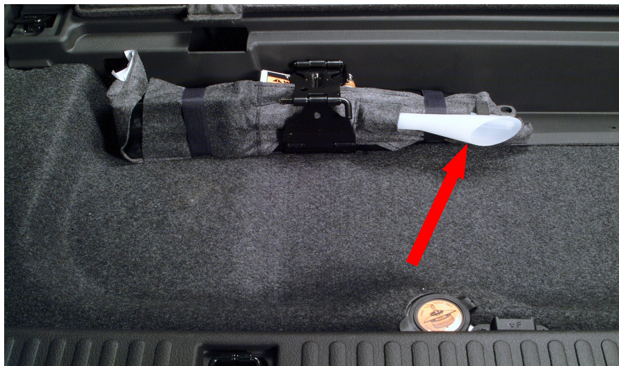
Figure 8. Fuel Funnel Location in Storage Bin
