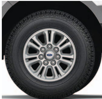
17" 7-lug aluminum Included with XLT Heavy-Duty Payload Package on XLT; Optional with Heavy-Duty Payload Package on XL (627)
