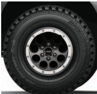
17" forged aluminum bead-lock capable Optional on SVT Raptor 64A
